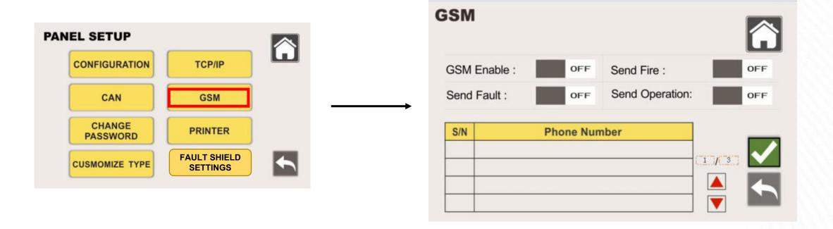
Next, set up "GSM", which is to send fire messages to mobile phones using 4G module.
