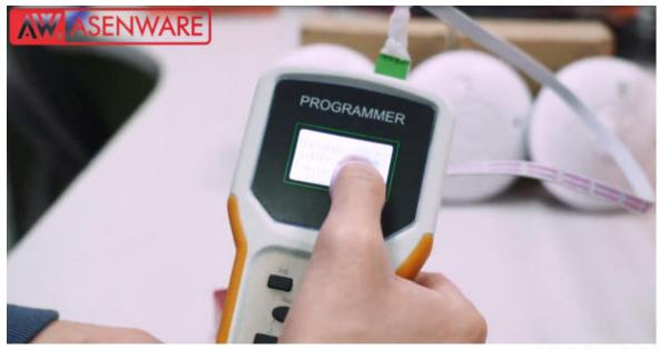
Connect the programmer connection cable to the connection port of the manual call point.
