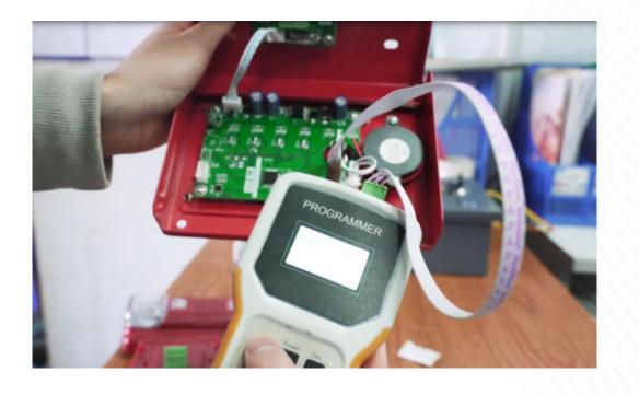
Connect the programmer connection cable to the connection port of the addressable annunciator.
