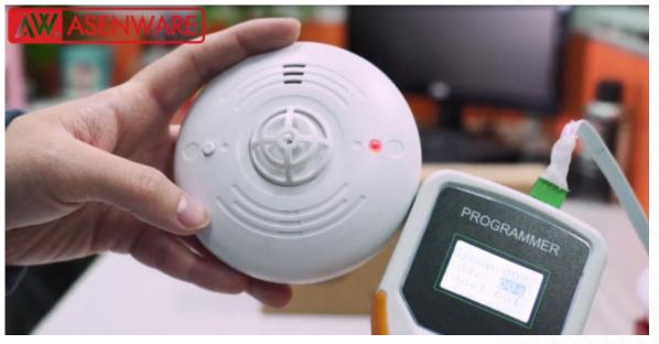
Press and hold the button of the combined detector to turn it on, after hearing a "beep", press and hold the button again to enter the programming mode. "Group: 001", "Panel: 001" remain unchanged, press
