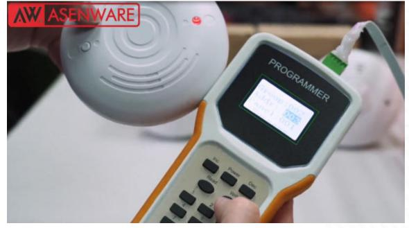
Press and hold the button of the smoke detector to turn it on, after hearing a "beep", press and hold the button again to enter the programming mode.
