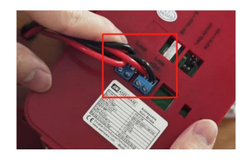
Connect the "LOOP OUT" wires of the manual call point base to the next product: addressable strobe sounder.
