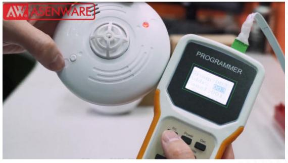
Press and hold the button of the heat detector to turn it on, after hearing a "beep", press and hold the button again to enter the programming mode.
