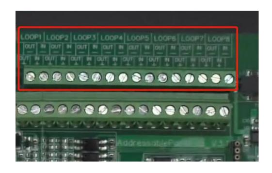
There are the wiring ports of 8 loops, and they are marked from LOOP 1 to LOOP 8 respectively.
